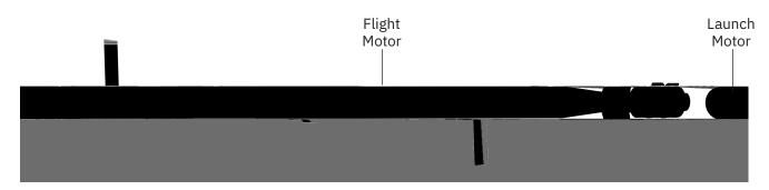
The Raytheon-produced Stinger missile is launched by a small launch motor that pushes it a safe distance from the operator before engaging the main flight motor. L3Harris provides both solid propellant rocket motors.
